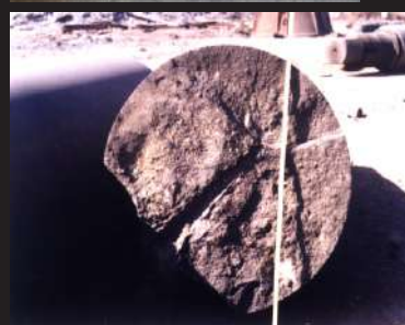
▲▲▲▲▲▲▲▲▲▲▲▲▲▲▲▲ Splitting Action Produced by a ThunderJet Charge on a 900 mm Diameter Steel Roller (left) and a 900 mm x 1400 mm Steel Ingot (right)
