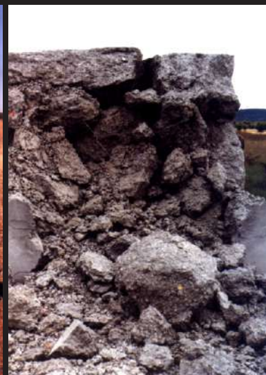
▲▲▲▲▲▲▲▲▲▲▲▲▲▲▲▲ A ThunderJet Charge and the Breakage Effect Produced by Blasting a Concrete Block Measuring 10.7 Cubic Metres
