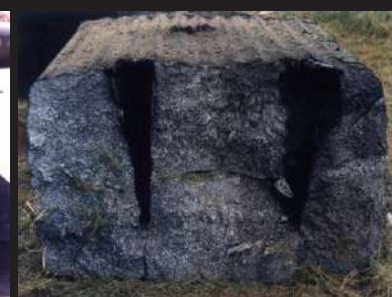
▲▲▲▲▲▲▲▲▲▲▲▲▲▲▲▲ Splitting Action Produced by a ThunderJet Charge on a 900 mm Diameter Steel Roller (left) and a 900 mm x 1400 mm Steel Ingot (right)
