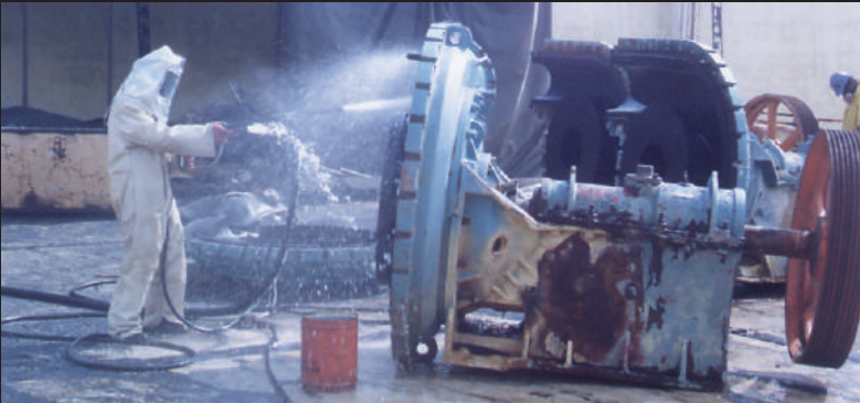
Decontamination of Radioactive Equipment Recovered from Uranium, Acid and Gold Plants
