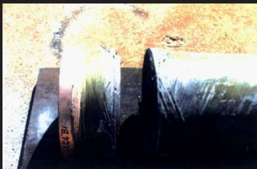
▲▲▲▲▲▲▲▲▲▲▲▲▲▲▲▲ A SabreJet Charge (20 g/m) Wrapped Around a Fibreglass Pipe (top) and the Resulting Cut After Firing (bottom)
