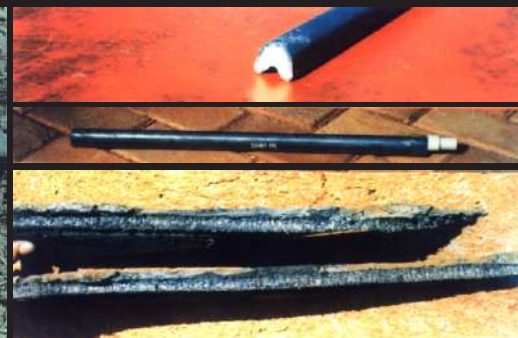
▲▲▲▲▲▲▲▲▲▲▲▲▲▲▲▲ A SabreJet Charge (400 g/m) From Two Different Views (upper and middle) and the Slicing Effect Produced on 25 mm Thick Steel (lower)
